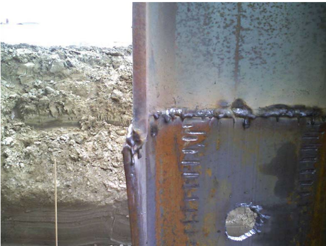
Misalignment, arc-strikes, unacceptable profile, contaminated surfaces, slag, undercut, porosity.
